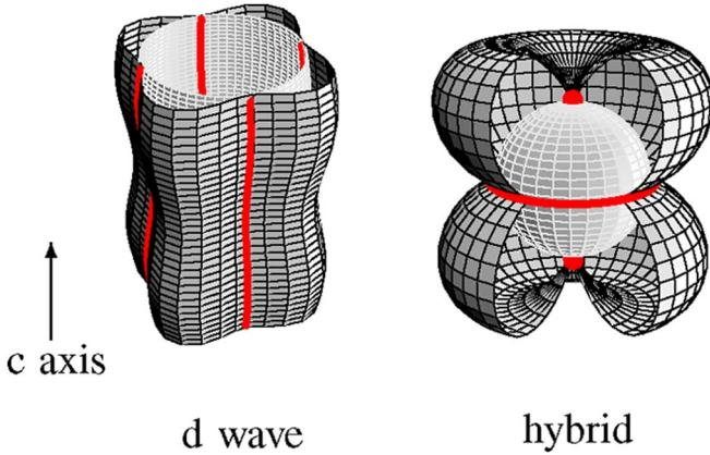
FIG. 2 (color online). Typical gap structures in tetragonal symmetry. Left:  $d_{x^2-y^2}$  gap on a (warped) cylindrical Fermi surface, with four vertical line nodes running along the  $c$  axis. Right: hybrid gap on a spherical Fermi surface, with one horizontal line node in the basal plane and two point nodes along the  $c$  axis.
