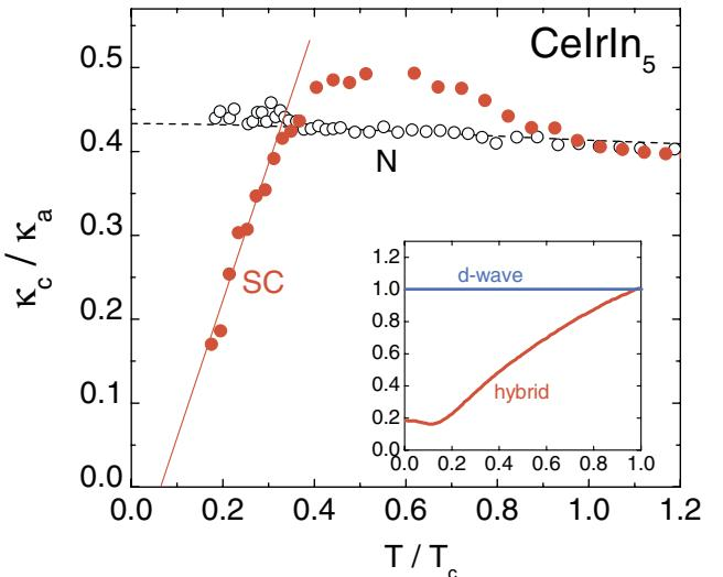
FIG. 3 (color online). Temperature dependence of the anisotropy ratio  $\kappa_c/\kappa_a$ , in the normal state ( $N$ ) and in the SC. The dotted line is the ratio of the two normal state fit lines in Fig. 1 and the solid line is a linear fit to the superconducting state data below  $T_c/3$ . Inset: calculated anisotropy (normalized at  $T_c$ ) for the gaps shown in Fig. 2, namely  $d$ -wave [26] and hybrid [19].
